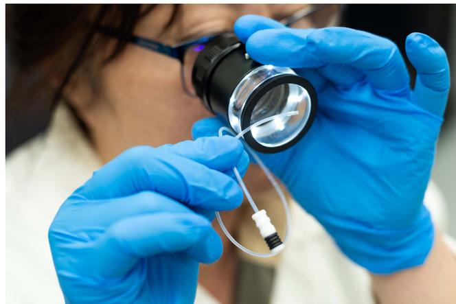
Check condition of Capillary Tubing
