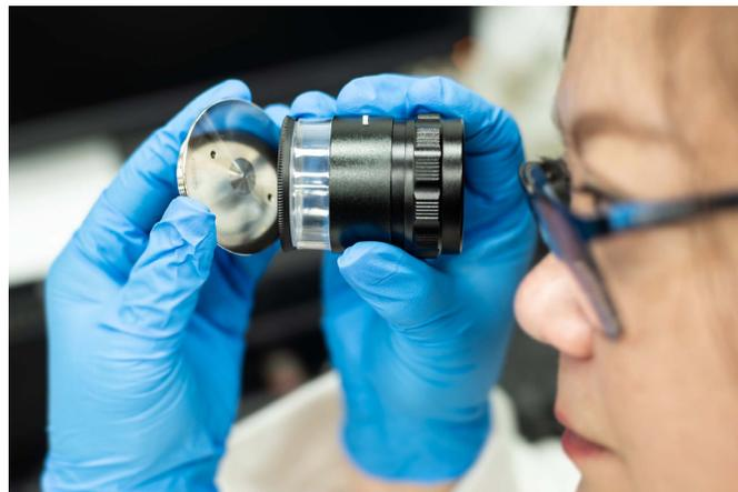
Check condition of ICP-MS Interface Cones
