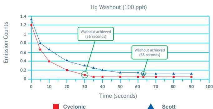
Figure 4. Washout times of 100 ppb Hg
