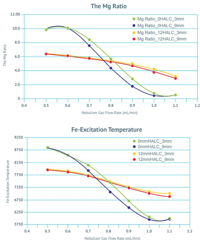
Therefore, the increase in sensitivity for both atom and ion lines can be attributed to the increase analyte loading to plasma when the nebulizer is inserted away from the aerosol impact zone and decrease sensitivity for ion lines can be attributed to the plasma cooling due to the increase nebulizer gas flow rates and water loading to plasma.
