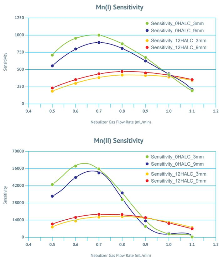
Figure 4 highlights the effect of nebulizer depth on Mn (I) and Mn (II) sensitivities as a function of nebulizer gas flow rate for two different height above the load coil (HALC) positions and two different nebulizer depths (3mm: closer to the aerosol impact zone and 9mm: away from the aerosol impact zone).
