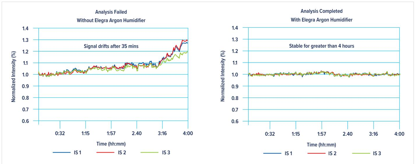
The graphs above demonstrate the benefit of using the Elegra with the real-world application of analyzing fusion samples with 0.5% lithium metaborate by ICP-OES. All three internal standard lines monitored began to drift quickly when no Elegra was used, while their responses were very stable with the Elegra installed.
