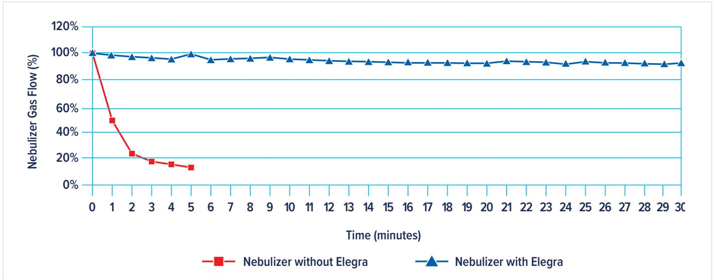
The graph above is the result of an extreme test, aspirating a 25% salt solution continuously without rinsing. Without the Elegra, the nebulizer begins to clog after only a few minutes as designated by the steep decrease in nebulizer flow. However, with the Elegra installed, the nebulizer is stable for well over 30 minutes.
