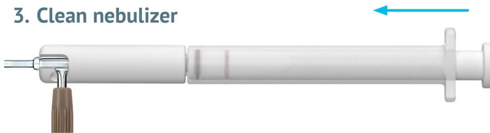
Particle build-up in a nebulizer capillary and tip causes sample flow to be constricted, thereby reducing nebulizer efficiency and performance. Now, blocked nebulizers can be safely and easily restored to optimum performance with the Eluo.
