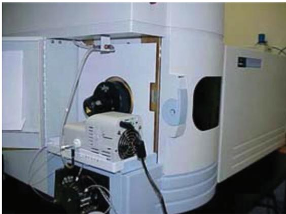
Figure 3. IsoMist mounted on the Optima 2100DV.
