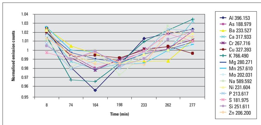
Figure 10. Long-term stability of 20 analyte wavelengths with the IsoMist at 25C.
